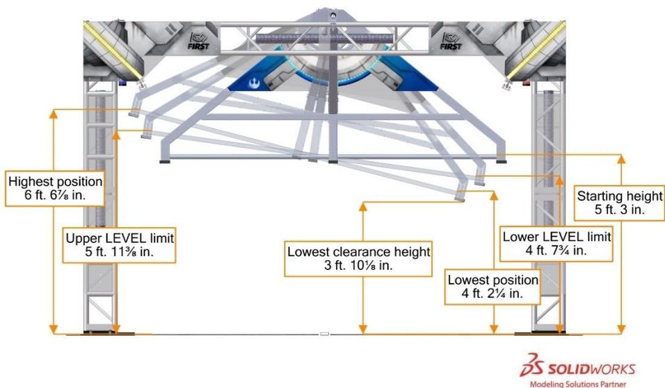
Figure 3-9 GENERATOR SWITCH range of motion.
