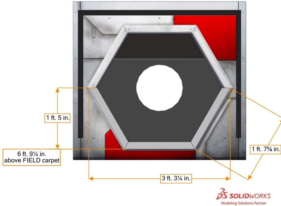
Figure 3-26 POWER PORT Vision Target
