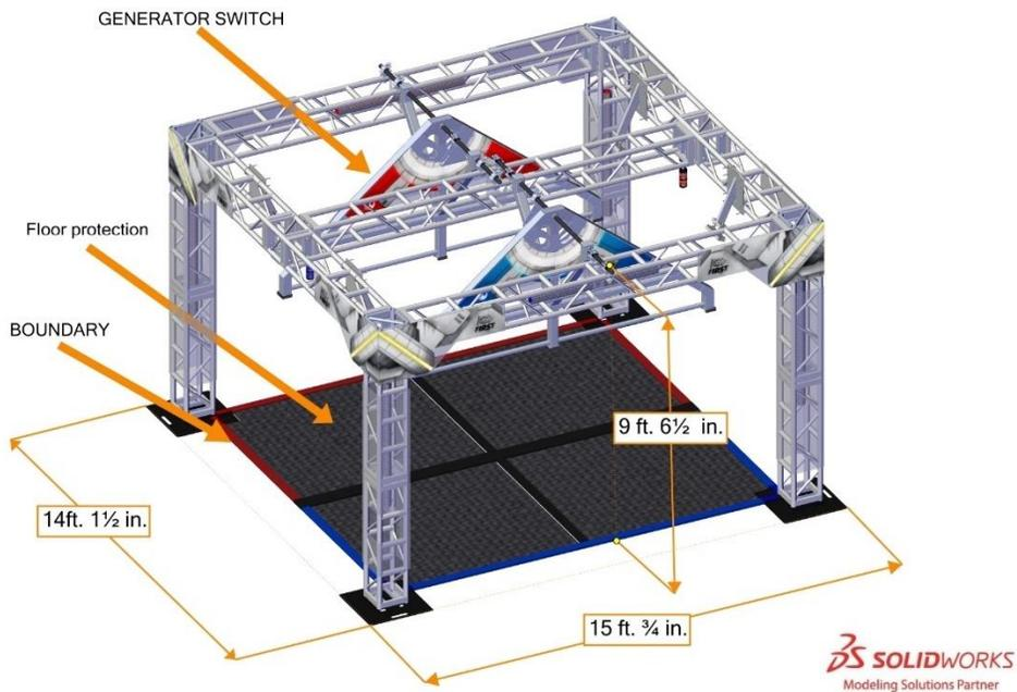
Figure 3-6 SHIELD GENERATOR
