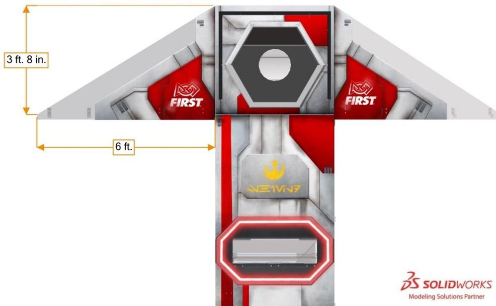
Figure 3-16 Backboard dimensions
